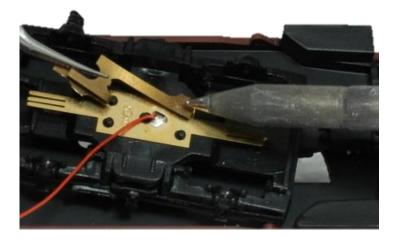
Insert the wires in the central hole of the current pickup, and lead them to the interior of the body. Pull them completely inside the body.
