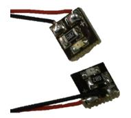
Glue the 2 Shine Micro R boards to the end wall of the carriage using a few drop of cyanoacrylate.
