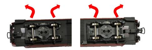
Insert the supplied current pickups on each of the boogies. Fit the 4 holes of the current pickup to the plastic pins of the boogie. A small drop of cyanoacrylate can be used to keep in place the current pickups.
