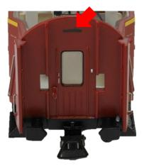
Drill a 2 mm hole in the back of the carriage in the center symmetry line of the wall.
