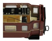
Please note the polarity of the capacitors, and connect them according to the Shine Plus manual. Cut the excess of the capacitors terminals.
