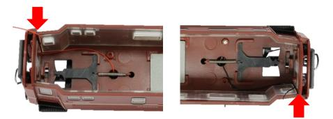
Before inserting the new wheels into the boogies, bend both sides of the current pickups in upper direction with a plier, as it can be seen in the illustrations below. This will ensure a proper contact to the axles.
