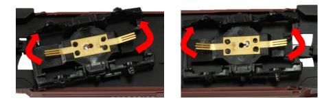
Insert 2 of the supplied new axles into each boogie.
