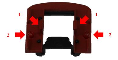
Level the light guides with a cutter to the same plane as the walls. Their surface can be adjusted/finished with a piece of fine sand paper.
