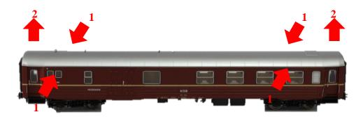
Some of the B3 carriages have interior walls up to the level of the carriage body, others (as the BF11 road number 21524, article 108.101, used in the illustrations) has interior wall up to the roof level.
