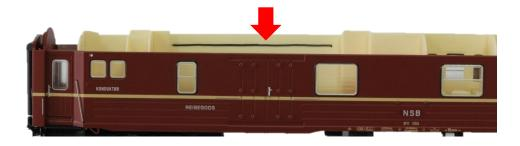
The interior is kept in place by 2 plastic pins at the end of the bodies (1). If the middle of the interior is pulled in upper direction (2), the pins will release the interior, and it can be removed easily.
