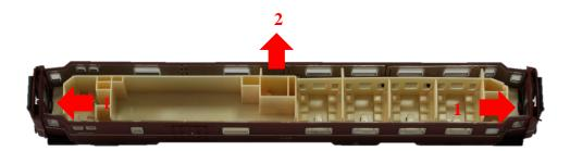
In most of the cases, the interior is glued with several glue drops to the body, so firmly movements will be necessary while removing it.
