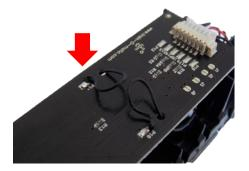
The wires from the axles in the motorized unit must be connected to the solder pads of the replacement board marked with P8 and P10. The solder pad marked with P9 can be left open.
