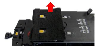
Cut a small piece of adhesive tape and label the 3 wires which connect the front lighting boards. You have to solder them to the replacement board in the same order.
