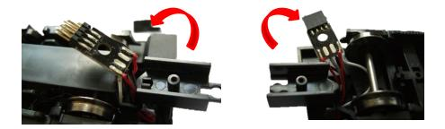
On both connectors are available 2 unused solder pads. These will be used to route the pickup shoe to the pcb. On the motorized unit solder a 10 cm long isolated wire to both solder pads, on the nonmotorized unit solder the wire connected to the pickup shoe to both solder pads. (Please note, on the motorized unit the connector is a pin type, on the non-motorized unit it has receptacles.)
