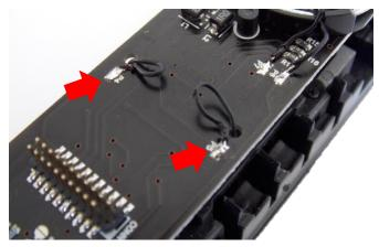
Insert the 4 pickup connection wire through the holes with the help of the tweezer and solder them to the board solder pads. Lay down the extra wires to the board.
