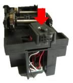
Check the fit of the connectors between the 2 units.
