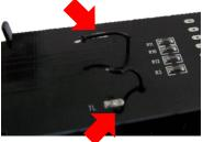
Connected to the current pickups in the AC version
