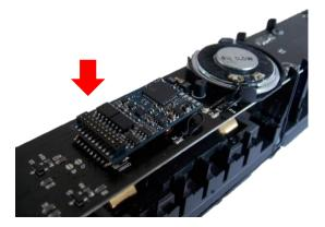
When assembling the housing, take care to arrange the wires to avoid their visibility from the outside. In the pickup wires area, on the insets (chairs) there are small adhesive black mask, which can be used to hold the wires in the proper position. In the cabin (cockpit) area, the wires which connect the front lighting boards can be tied together, and in this way they will be invisible from the outside.
