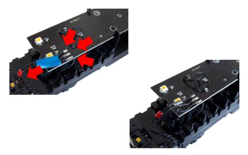
Place over the LEDs the adhesive black mask (take care to fit the openings exactly over the 2 LEDs). Lay it and press over the complete surface to ensure that it sticks to the board.
