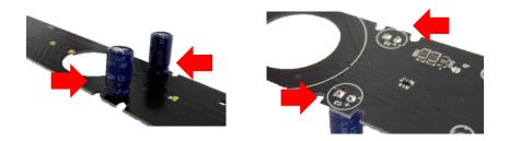
Fit the speaker housing in the bottom of the new board. Take care to match the 2 plastic dowel pins of the speaker housing to the holes in the board.
