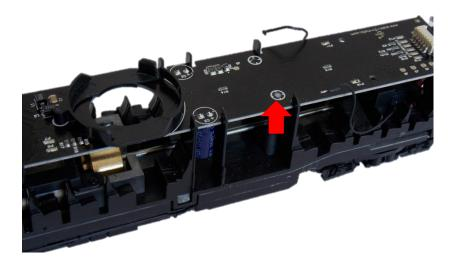
and fasten it with the 2 screws. Two dovel pins of the body will guide the positioning of the board in the base.
