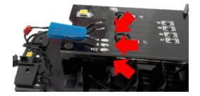
The solder pads of the replacement boards are situated in the same location as on the originals, so the positioning of the wires on the replacement board is straight forward.
