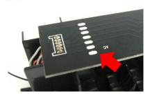
Connection of the power pickup shoe in the non-motorized unit
