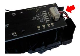
Place the speaker in the holder and solder the wires.
