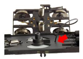
Insert the two washers contained in the package over the screw before fixing the boogie. Depending on the screw size, the internal diameter of the washers may need minor adjustments. This can be done using a small file.
