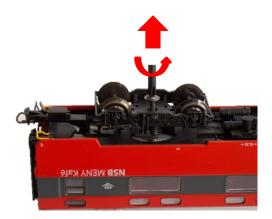
While removing the boogie from the carriage, preserve the 2 springs and the screw for later use.
