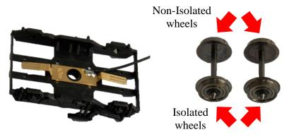
Insert the 2 axle pairs back to the boogie. On each boogie, the isolated wheels must be on the same side, and on the two boogies they are mirrored. Only with this wheel arrangement is possible to collect both polarities of the DC/DCC signals from the track.
